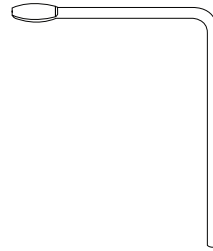
EBM-32: Chuck Release Key (1)
