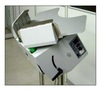
(3) When using the paper tray while setting it horizontally, load sheets of paper little by little (If the paper is loaded in mass, the tray receives the weight all at once, which makes it difficult to jog the paper properly).
