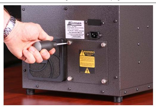
4) Loosen the (4) screws from the Voltage Selection Panel and remove the Voltage Selection Panel.
