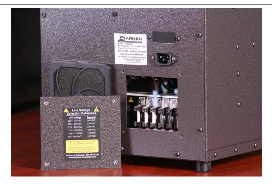
5) Using the Line Voltage Selection Reference label on the Voltage Selection Panel, confirm the correct jumper setting for the outlet voltage noted in Step 3.
