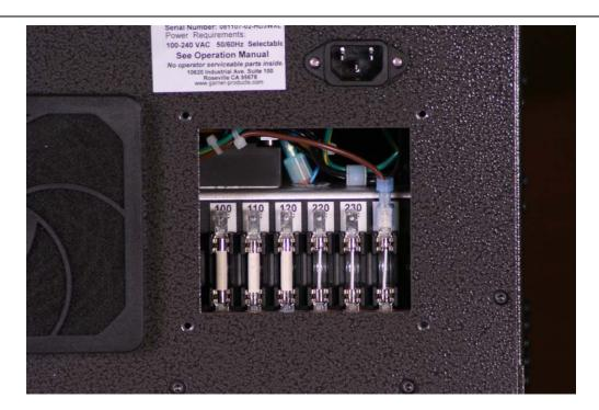
Notice, this photo shows the correct jumper setting for 240 VAC.
