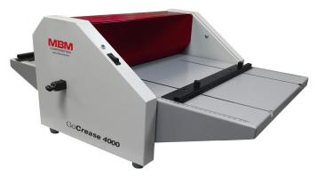
This creasing and perforating machine with a working width of 17.7" is designed for the final processing of graphic materials up to 16.5" x 23.4". Creasing enables high-quality folds of digitally printed paper. The machine can also be controlled via a foot pedal. The GoCrease™ 4000 is built with high quality anvil perforation, as well as 3 different creasing channel widths.
