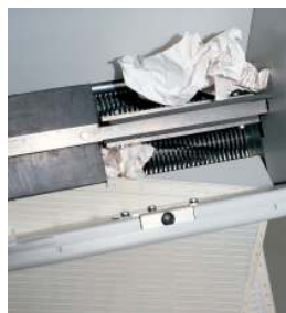
Automatic mechanical feeding system with revolving flaps
