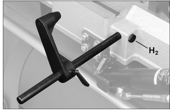
Figure 6-7: installing work stop (712 only)
