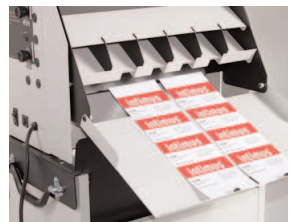
Fig. 8 First pass stacking
