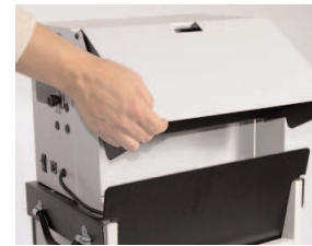
Fig. 13 Lifting the rear assembly
